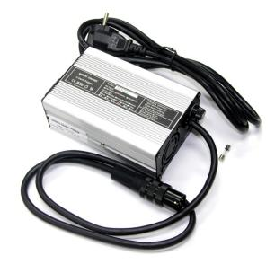
The GS8001 MKII single bay charger is designed to quickly and efficiently charge / recondition BB-2590/U batteries and compatible models. The charger is fitted with a durable aluminum casing, LED status indicator and is protected against reverse polarity charging and short circuits. The GS8001 MKII is an intelligent charger which varies the charging stages for optimal charging and reconditioning of BB2590/U batteries.
